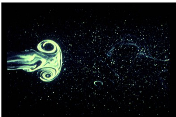
LIF snapshot showing dye concentration within a vortex ring
